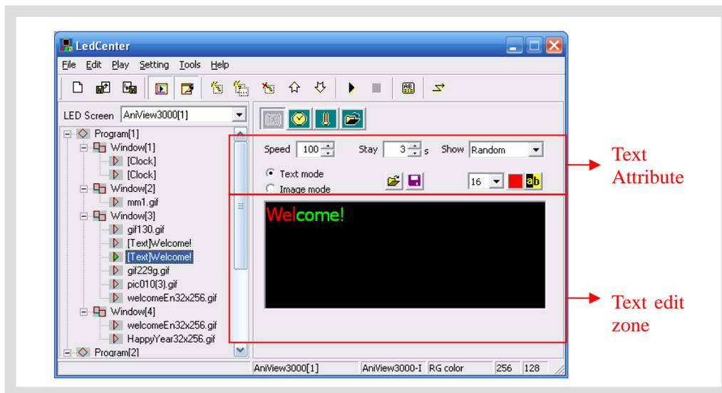
Figure18 Text program (text mode) edit interface
